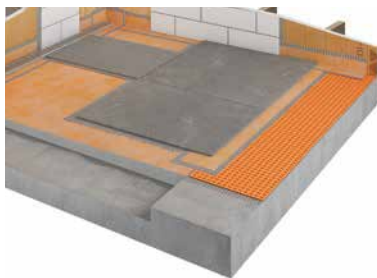
Recessing the Shower Floor
