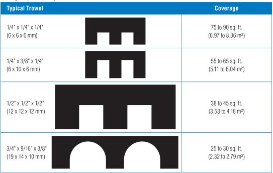
\*\*\* Trowel dimensions are width/depth/space. Actual coverage will vary according to substrate profile and tile type.
