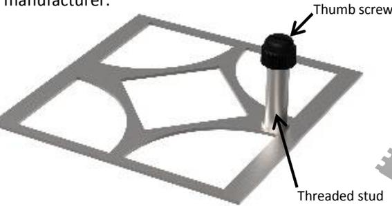
**Warning:** Each threaded stud is covered with a plastic thumb screw to prevent thin-set mortar from corrupting thread. Do not remove until after grouting.
