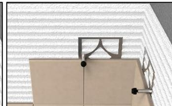
**Note: System will not work on tile thicknesses less than 5/32" or greater than 1/2"**
